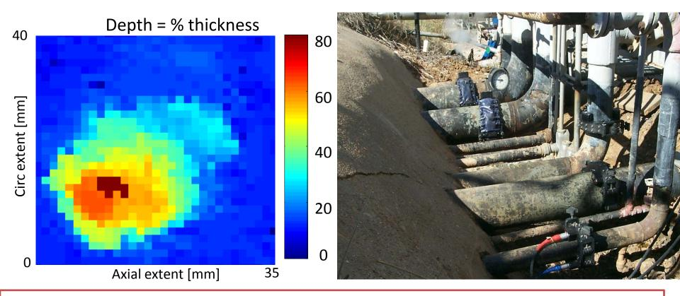
The purpose of this work is to analyze the effect of the shape of a defect on the Reflection Coefficient (RC) spectrum to find a method for remote sizing of defects.
