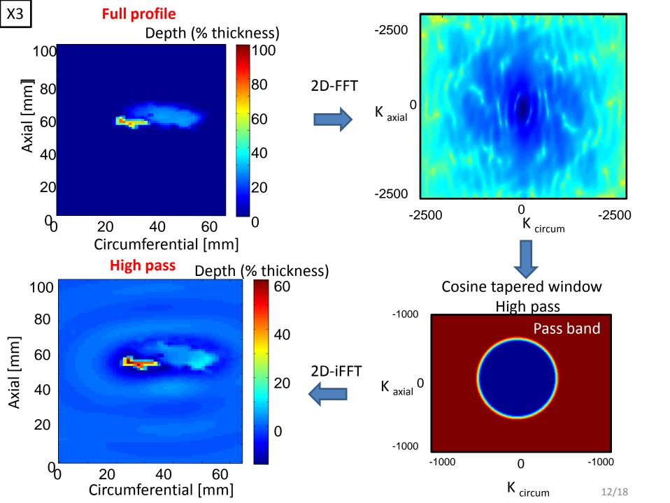
The original profile can be reconstructed by the superposition of the two defect matrices
